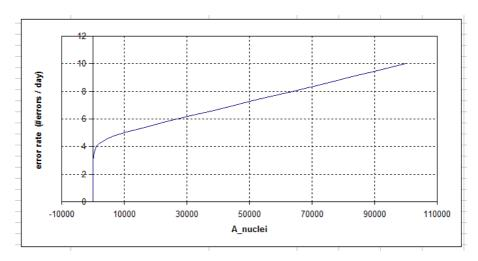
**Figure 2**. A close study of the results of the experiment may reveal a simple relation between the error rate and the rate of primary nuclei of CR. In this hypothetical example the relation is a linear one.
